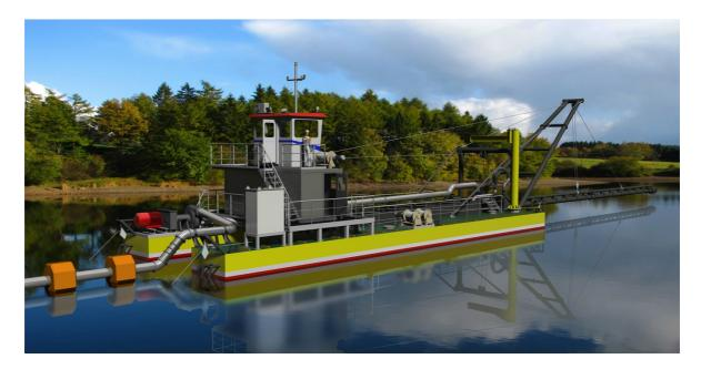
The PSD350 Plain Suction Dredger is designed for dredging inland lakes, up to -40 m below water level. Reduced dredging depth can be achieved by reducing the length of the lower dredge pipe.
