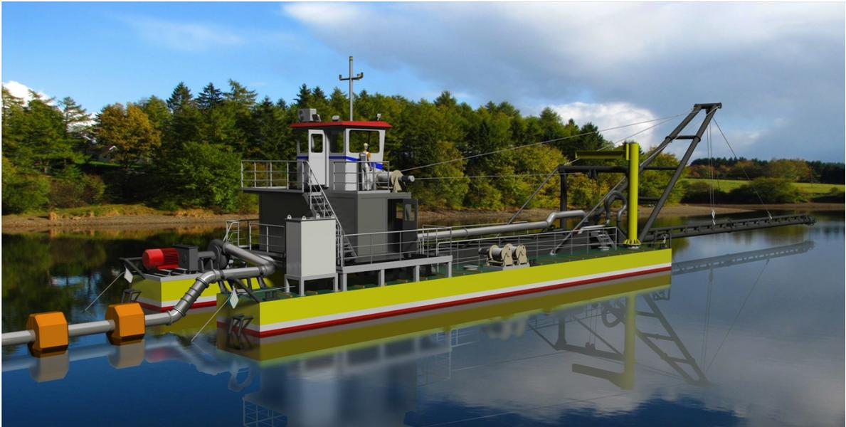
The PSD350 Plain Suction Dredger is designed for dredging inland lakes, up to – 40 m below water level. Reduced dredging depth can be achieved by reducing the length of the lower dredge pipe.
